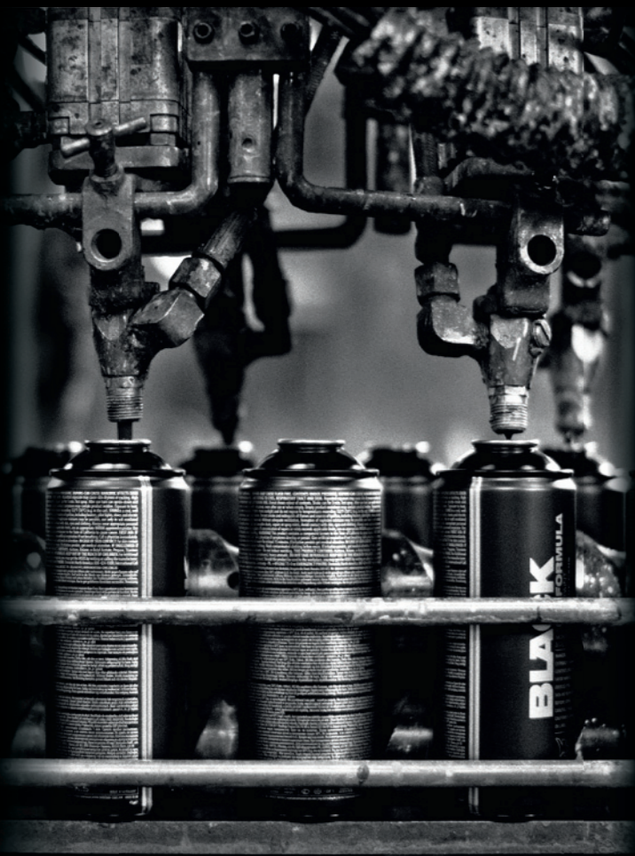
Production of the Montana BLACK series in Haßmersheim Germany, Filling line.
